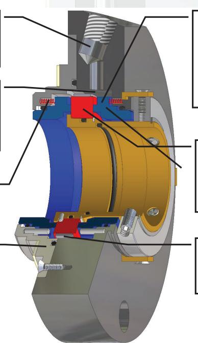
Self-aligning stationary design handles stuffing box misalignment with a single movement vs. oscillating springs in rotary designs (1 movement vs. RPM x 2 for spring
