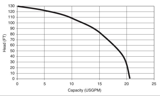
EBG2-21 (2HP) Synchronous Speed: 3450 RPM 11/4 inch Discharge
