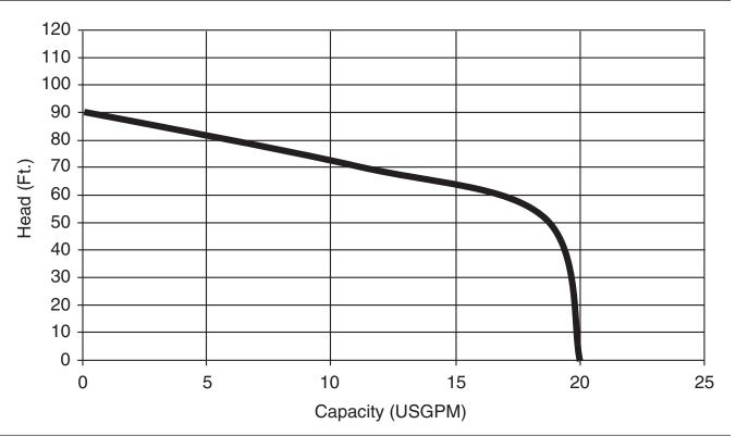
EBG2-212C (2HP) Synchronous Speed: 3450 RPM 11/4 inch Discharge
