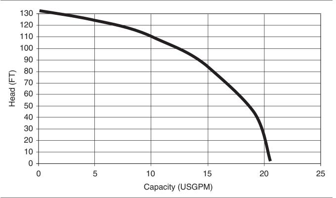
Synchronous Speed: 3450 RPM 2<sup>1</sup>/<sub>2</sub> / 3 inch Discharge EBG-31 (3HP)
