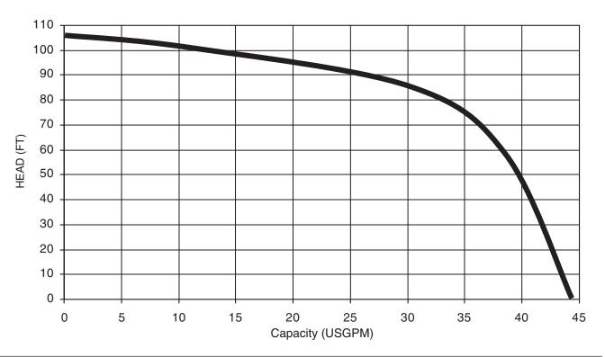
EBHG2-21 (2HP) Synchronous Speed: 3450 RPM 1<sup>1</sup>/<sub>4</sub> inch Discharge
