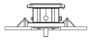
9. Mount the drive magnet assembly (740B) onto the drive shaft so that the driver cams engage. Secure the drive magnet assembly using the lockwasher (382) and capscrew (791D).
