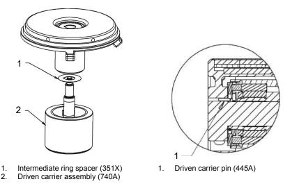
Place the driven magnet assembly (740A) on the workbench, and then mount the pre-assembled bearing cartridge (849) and backplate (444) assembly onto the driven magnet assembly from above. Make sure the driven carrier pin or key (445A) engages the carrier groove in the bearing cartridge (849).
