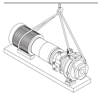
Figure 2: Proper lifting method for a pump with a base and driver
