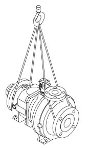
Figure 1: Proper lifting method for a bare pump
