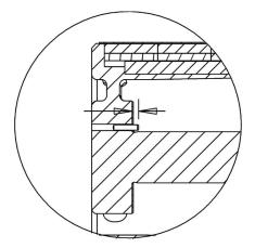
4. Cut out a small notch on the inside diameter of the intermediate ring gasket (351X) in order to create a recess for the driven carrier pin (445A) or key, depending on size.
