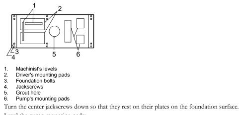
5. Level the pump mounting pads:
