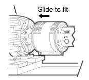
10. Use a nut, a bolt, and two washers to secure the coupling guard halves together.
