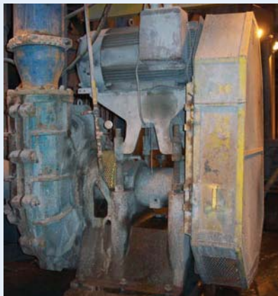
SRL-XT 14x12-36 on Ball Mill Discharge Service
