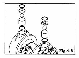
• Remove the O ring, valve seat, ball and valve stopper. [Fig.4.8]
